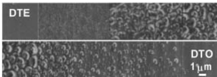
**Figure 7.** Shown above are a series of twelve 5 mm \_ 5 mm AFM phase images from a compositional gradient of DTE/DTO blend film fully annealed for 16 h.
