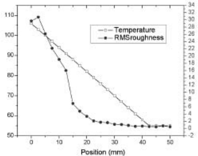
**Figure 6.** A plot of temperature and RMS roughness vs. position shows both the linearity of the temperature gradient and the distinct drop in RMS roughness that occurs near 90 °C which happens to be the glass transition temperature of DTE (91 °C).
