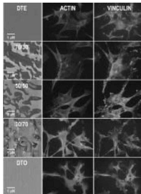
**Figure 2.** From top to bottom are five 5 mm × 5 mm AFM images in which the amount of DTO is increasing. The discrete DTE/DTO blends form phase-separated domains under the prescribed annealing conditions. Immuno-fluorescent staining for actin and vinculin of MC3T3-E1 osteoblasts showing the cytoskeleton and focal adhesion contact formation 16 h after seeding on each of the respective homopolymers and blends.
