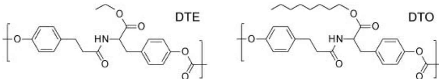
**Figure 1.** Synthetic scheme and chemical structure of desaminotyrosyl-tyrosine alkyl esters and the resulting polycarbonates. The pendant R groups of the polycarbonates reported in this article consist of ethyl and octyl esters, respectively. The corresponding polymers are referred to as poly(DTE carbonate) and poly(DTO carbonate).
