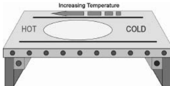
**Figure 4.** The gradient hot-stage shown above consists of an aluminum (Al) sample plate. Two adjustable Al blocks, with machined heating/cooling channels, are attached to the bottom of the plate. The block channels hold cylindrical heating cartridges or accommodate plumbing for fluid-mediated cooling. The range and slope of the temperature gradient are tailored through the respective block temperatures and their distance apart.
