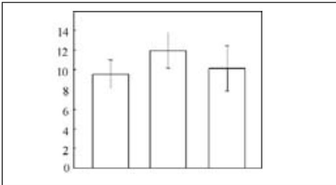
**Figure 1.** Strength of CPC-suture fiber composite made by three different operators to examine operator sensitivity. The three operators produced cements with similar strengths, indicating that the composite fabrication method was reproducible. Horizontal line indicates values not significantly different ( $p > 0.05$ ).
