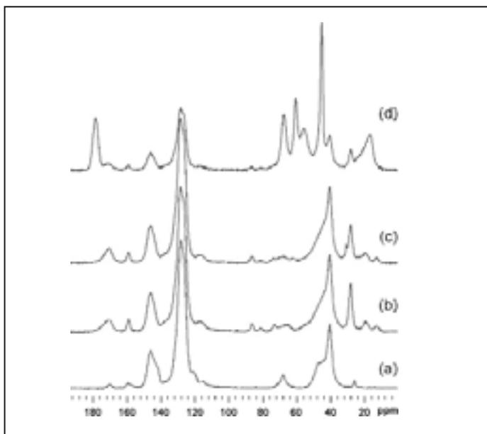
**Figure 1.** The solid state  $^{13}\text{C}$  NMR spectra of Fmoc-glycine Wang resin (a), GR(Pbf)GD(Obut)S(But) Wang resin (b), GR(Pbf)GD(Obut)S(But)-initiator Wang resin (c), R(Pbf)GD(Obut)S(But)-poly(HEMA) Wang resin (d).
