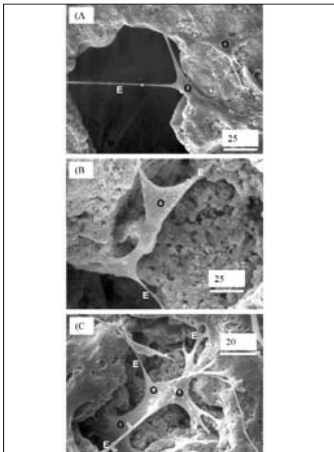
**Figure 4.** SEM showing osteoblasts migrating into the macropores of a CPC scaffold. “O” = osteoblasts, “E” = cytoplasmic extensions. (A) Osteoblast cell attached near the edge of a macropore. (B) Cells migrated into macropores. (C) Cells colonized on the pore.
