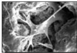
Scanning electron micrograph showing osteoblasts migrating into the macropores of a calcium phosphate cement scaffold where cells are colonized on the pore bottom and established cell-cell junctions. From: Hockin H. K. X. et al., Strong, Macroporous and In-Situ Hardening Hydroxyapatite Scaffold For Bone Tissue Engineering.
